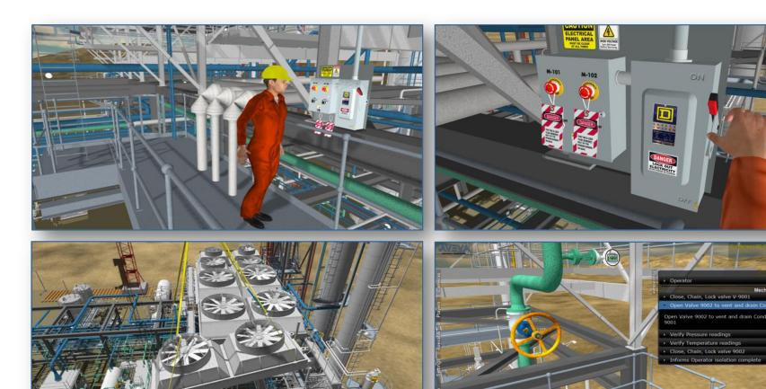
Sample Application demonstrating a Multi-User 'Lock-Out / Tag Out' activity for removing a condenser
